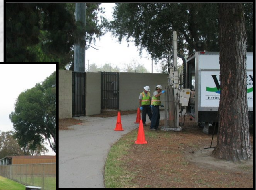
B-124 Hydropunch Groundwater Sampling
